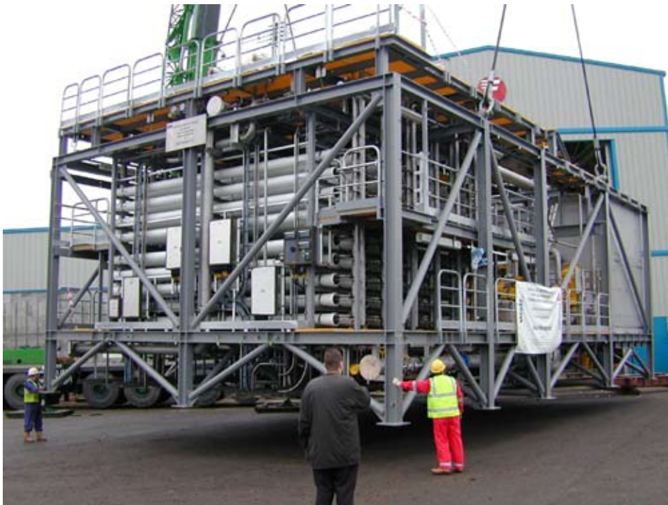
FIGURE 12 Modular sulphate removal unit for an FPSO.
