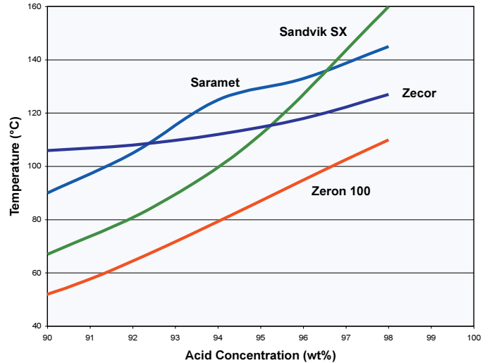
FIGURE 2 Iso-corrosion curves (0.1mm/y) in strong sulphuric acid
