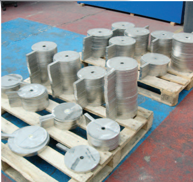
Figure 7 ZERON 100 orifice plates being prepared for shipping.
