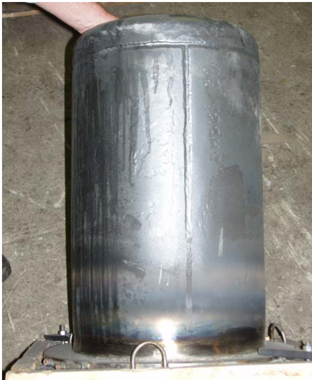
Retort used at 2200°F, welded with alloy 82 (ERNiCr-3) wire. Weld bead heavily oxidized.
