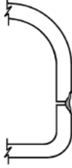
thin by oxidation after long 2000°F service
